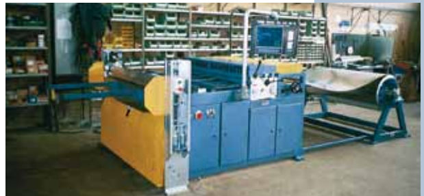
Automatic rectangular duct forming machine type KA 1500 Shopmaster.
