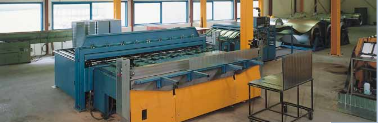
Automatic rectangular duct forming machine type KA 1500-3000
