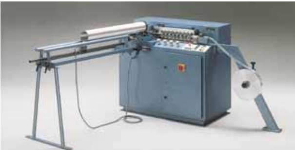
Automatic flexible duct forming machine TS 580
