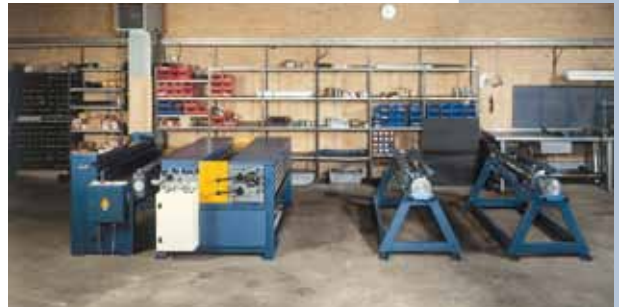
Feeder for plasma cutting system. FE 1500-2000
