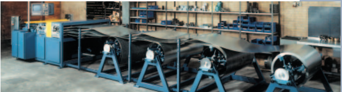
Automatic rectangular duct forming machine type KA 1501 A4.
